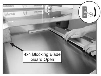
**Figure 50.** Adjusting fence perpendicular to the blade.
